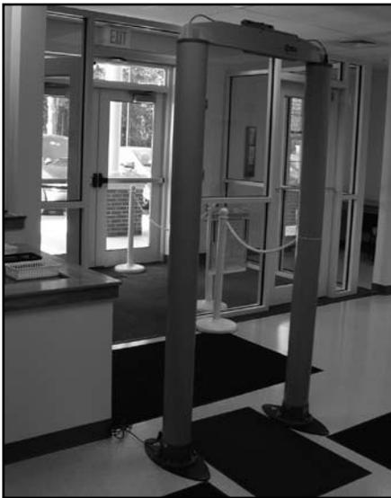
**Security at front entrance:** The entrance security was designed to easily accommodate a person with a disability through the positioning of the security gate and by lowering the bailiff's transaction counter
